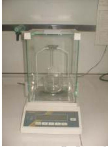
108 Fig.2. Experimental apparatus for the apparent density determination installed with a 109 precision balance. 110 111
