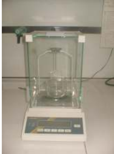
Fig.2. Experimental apparatus for the apparent density determination installed with a precision balance.
