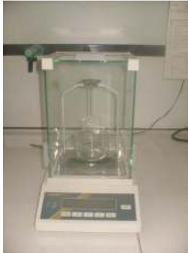
113 **Fig.2. Experimental apparatus for the apparent density determination installed with a**
