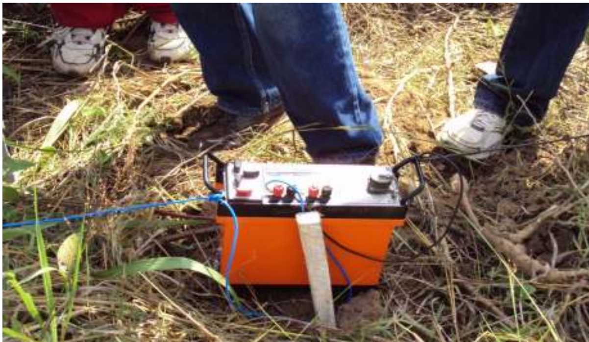
Figure 4: The versatile ABEM SAS 4000 – High resolution resistivity meter. Positioned at probe point.
