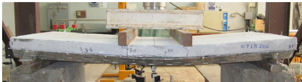
Fig. 14. Crack pattern for tested specimen (0.7 LS 200)
