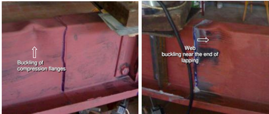
Fig. 12. Mode failure of test series (C)
