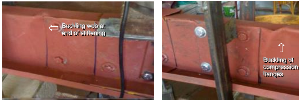
Fig. 9. Mode failure for specimens (D240-1, and D240-2)
