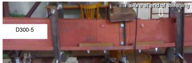
Fig. 10. Mode failure for specimen (D300-5)
