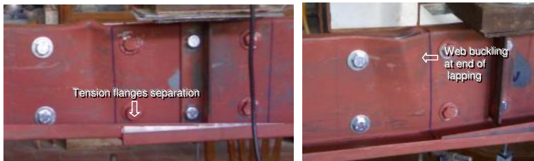
Fig. 11. Mode failure for specimens (D240-3 and D240-4)
