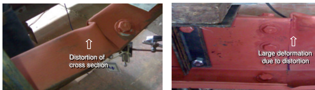
Fig. 8. Mode failure of test series (B)
