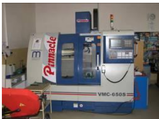
109 Fig. 3 Vertical machining centre for experiment
