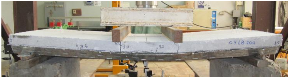
Fig. 14. Crack pattern for tested specimen (0.7 LS 200)
