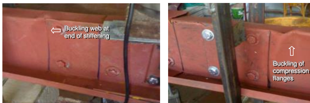
Fig. 9. Mode failure for specimens (D240-1, and D240-2)
