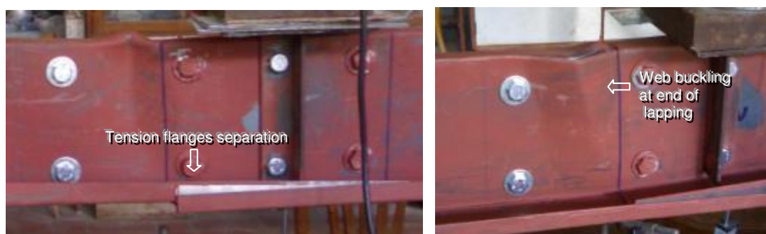
Fig. 11. Mode failure for specimens (D240-3 and D240-4)
