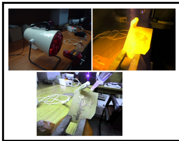
Fig. 2: Temperature control using IR lamp set up.
