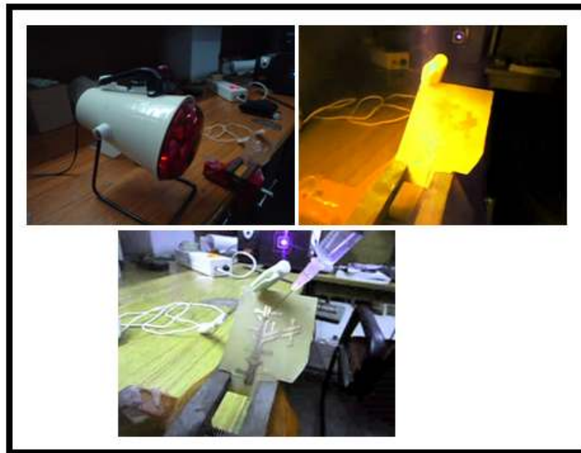
Fig. 2: Temperature control using IR lamp set up.
