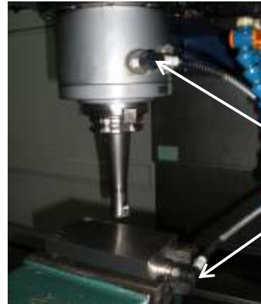
110 Fig. 3 Vertical machining centre for experiment and detail with sensors
