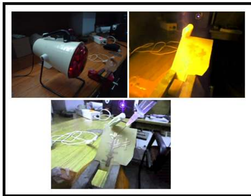
Fig. 2: Temperature control using IR lamp set up.
