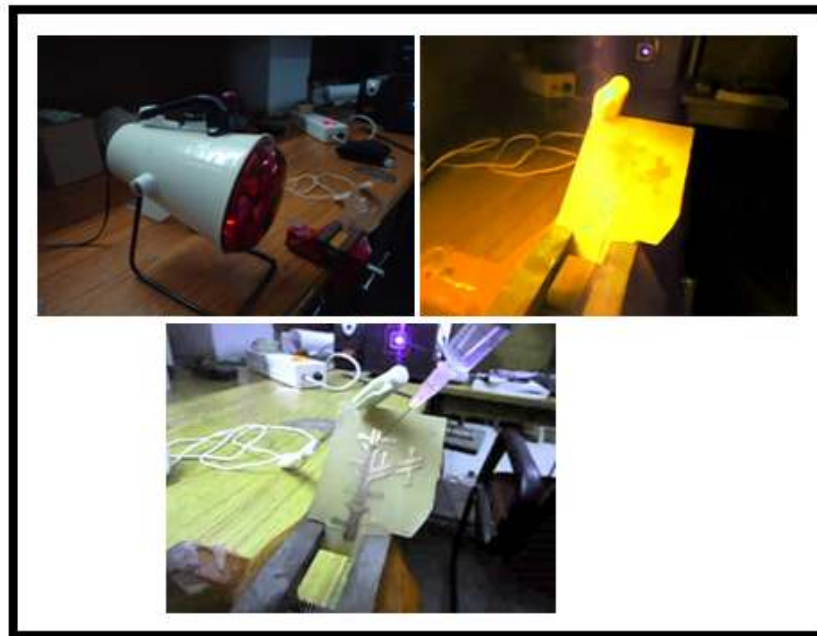
Fig. 2: Temperature control using IR lamp set up.
