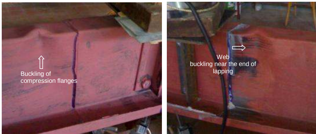
Fig. 12. Mode failure of test series (C)
