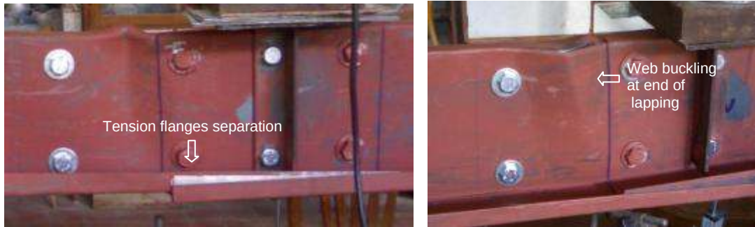
Fig. 11. Mode failure for specimens (D240-3 and D240-4)
