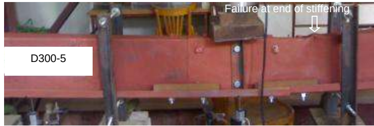
Fig. 10. Mode failure for specimen (D300-5)
