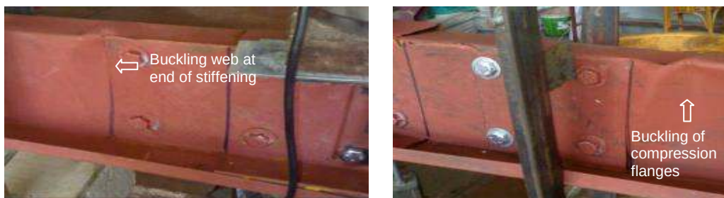
Fig. 9. Mode failure for specimens (D240-1, and D240-2)
