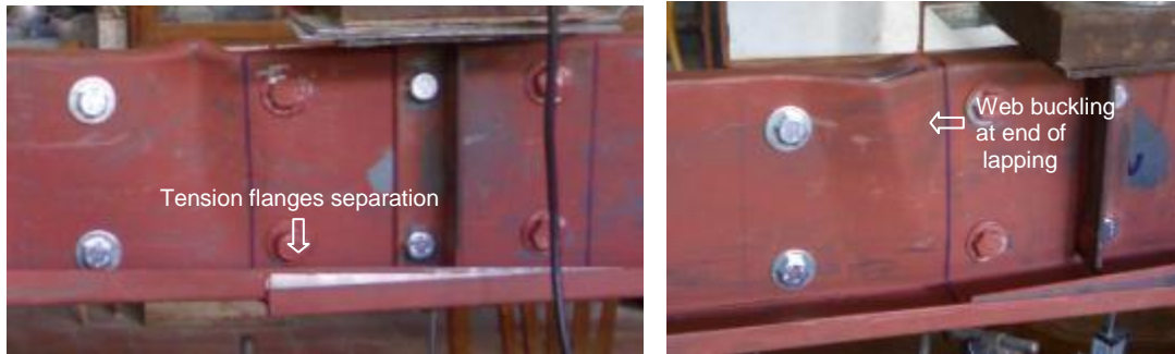
Fig. 11. Mode failure for specimens (D240-3 and D240-4)
