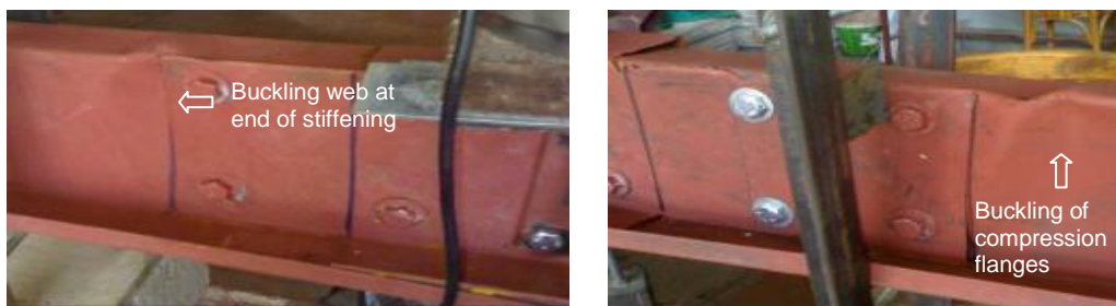
Fig. 9. Mode failure for specimens (D240-1, and D240-2)
