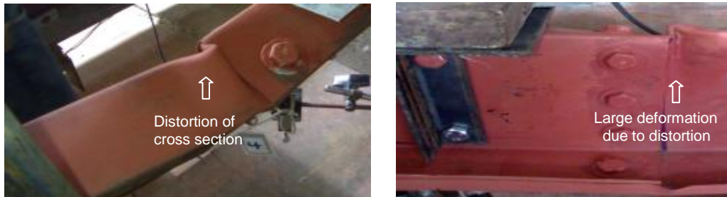
Fig. 8. Mode failure of test series (B)
