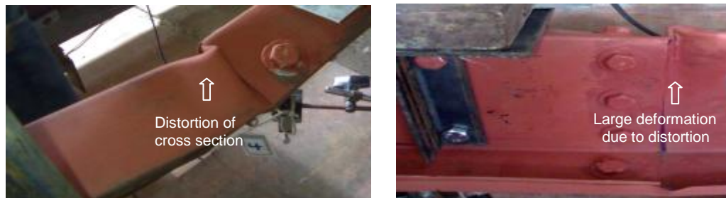
Fig. 8. Mode of failure of specimens' series (B)
