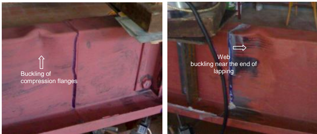
Fig. 12. Mode of failure of specimens' series (C)
