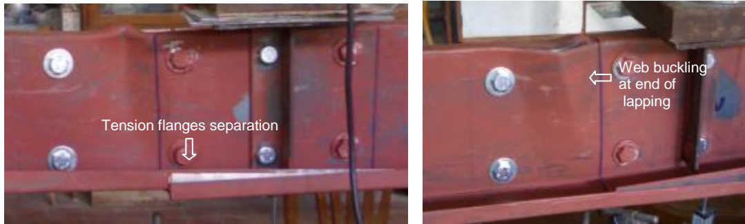
Fig. 11. Mode of failure of specimens (D240-3 and D240-4)
