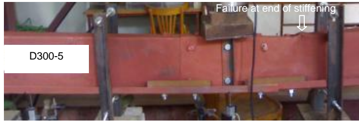
Fig. 10. Mode of failure of specimen (D300-5)
