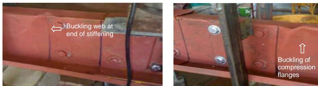
Fig. 9. Mode of failure of specimens (D240-1 and D240-2)
