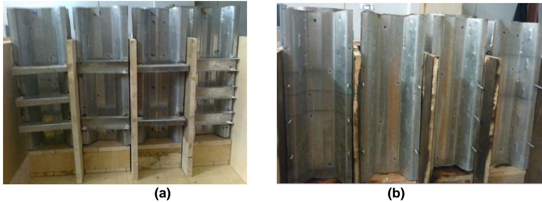
Fig. 4. Specimens enhanced with cold formed members (U, C) (a) and enhanced with Self-drilling screws (b).
