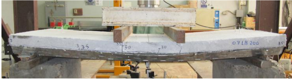
Fig. 14. Crack pattern for tested specimen (0.7 LS 200)
