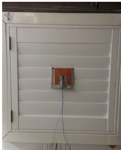
83 Fig. 4. Heat flux sensor fixed on back of a panel
