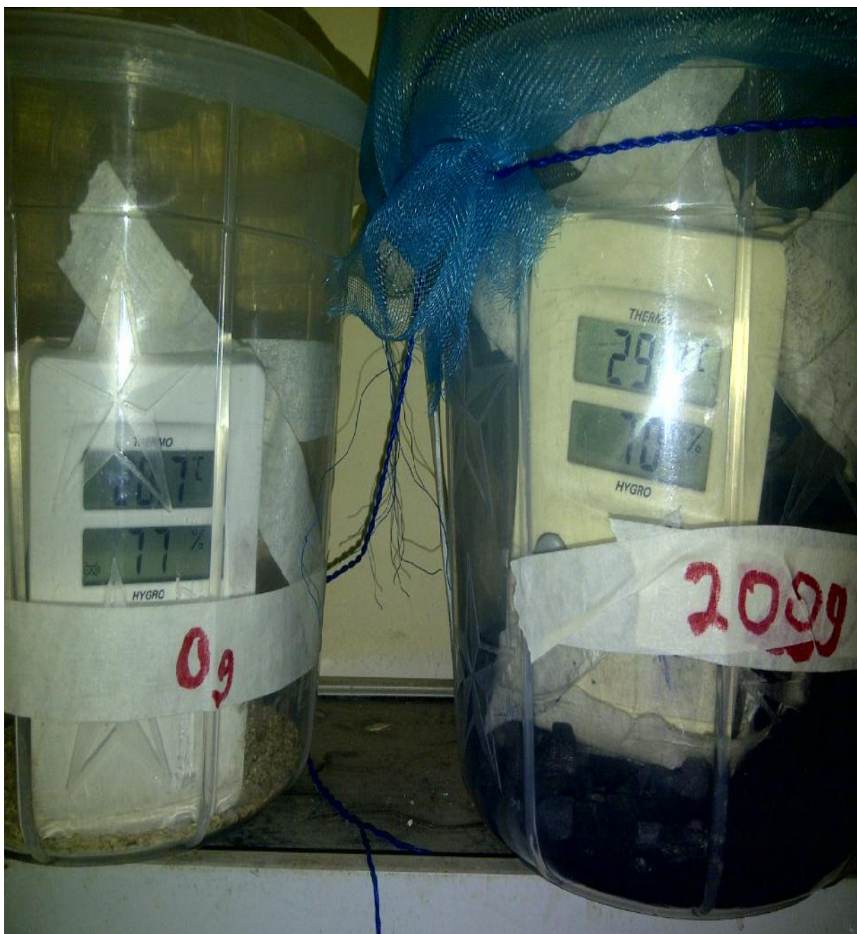
Plate 4. Differential storage conditions (relative humidity) of the control and highest charcoal desiccant treatments of stored sesame seed.
