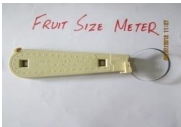
Figure 1c: Fruit size meter used to determine the fruit diameter regularly on weekly basis.
