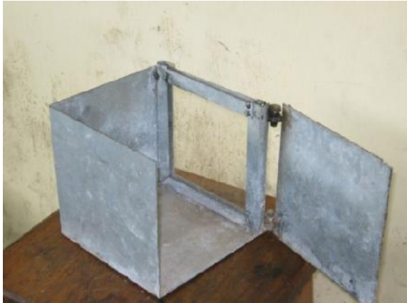
Figure 1: Angle of repose measuring box for freshly grated mash
