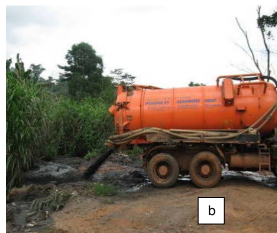
Fig. 1. Partial view of two types of faecal sludge disposal systems at Nomayos, Yaounde. (a) discharge into a well, (b) direct discharge on the ground.
