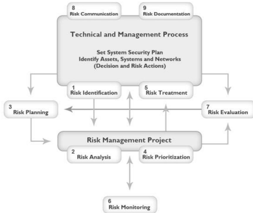
Fig. 5. Risk management framework for the smart grid.
