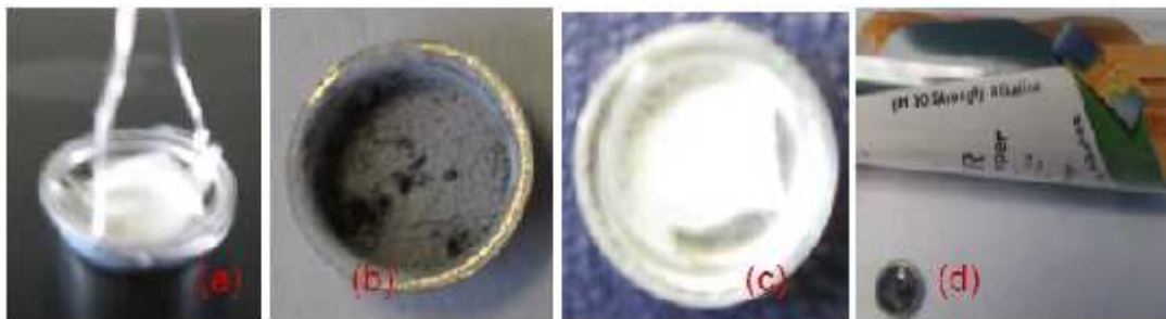
288 Fig 6. Thermogravimetric analysis: (a) pan loaded with 12 mg of LEG, (b) the remains after 289 heated to 600°C; (c) the products at 800°C, (d) alkaline pH of the aqueous solution of the 290 ashes. 291
