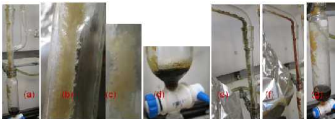
Figure 3. Step-by-step illustration of decomposition process of LEGs (a) Solids deposited in the condenser, (b) and (c) Magnification of selected sections of (a), (d); crystallization of solids in the collection funnel, (e) deposit of greenish solids, (f) deposit of reddish solids, (g) deposit of yellow solids
