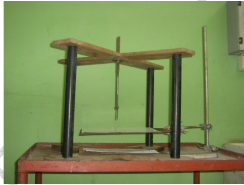
Fig. 6: Electrode Stand T_G with the barrier carrier.
