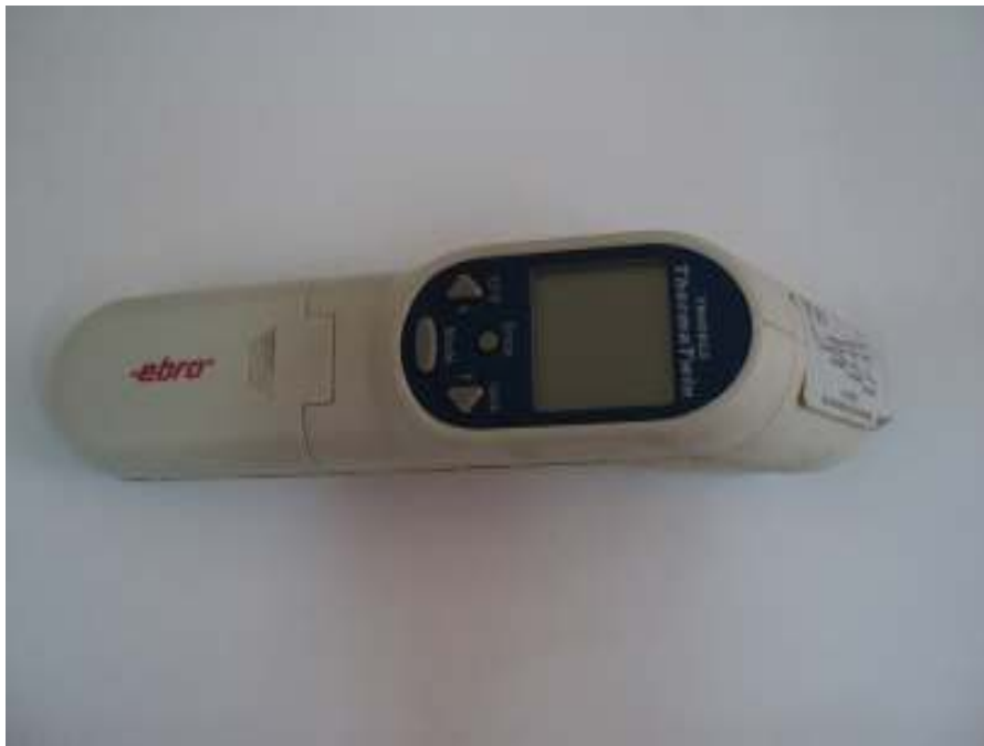
A – Germany Non Contact Temperature measuring Device
