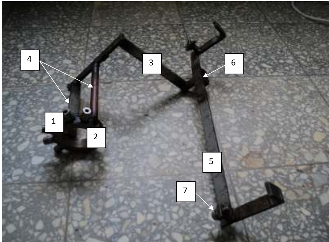
Figure 1 Cutting Fluid two-way/multiple feeding device for Turning Processes.
