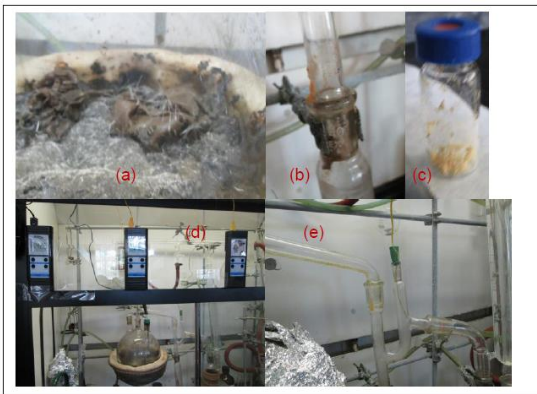
Fig 2. Step-by-step illustration of the decomposition process of LEGs: (a) the white needle shaped crystals grown in tope of the cold residues; (b) accumulation of solids out of the joints; (c) a sample of the solids; (d) the setup; (e) the condenser with solids.
