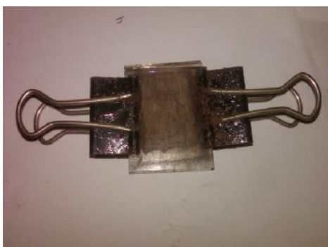
Figure 3: assembled solar cell
