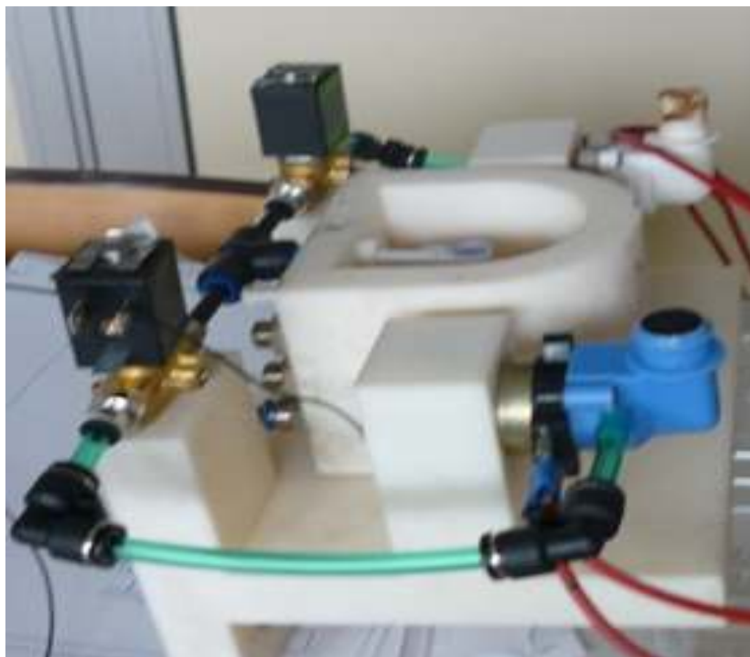
Figure 5: thermo-chemical device using pumps for spraying
