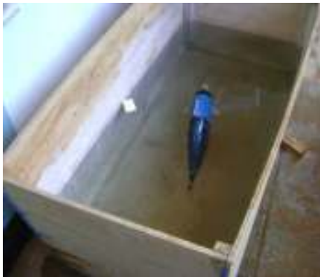
243 Fig. 6 Wooden box for testing the robot bump sensor. The robot is made to swim inside it in 244 a tight circle 245
