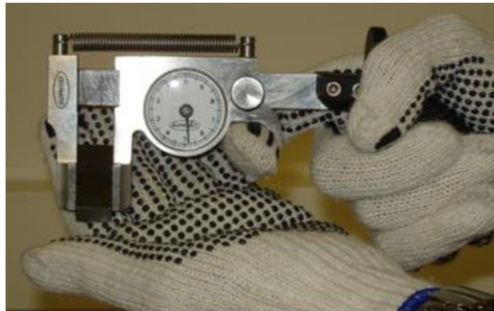
Fig. 2. Analog calliper during the calibration process.
