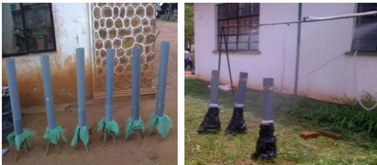
Figure 3: (a) constructed leachate extraction columns; (b) simulating rain on the leachate extraction column
