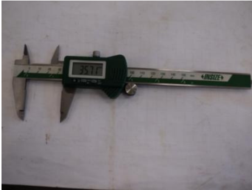
Fig. 2.2 - Insize Digital Vernier Caliper
