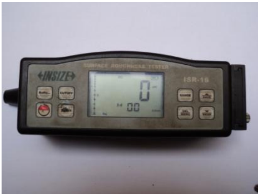
Fig. 2.3 - Insize Surface Roughness Tester ISR 16
