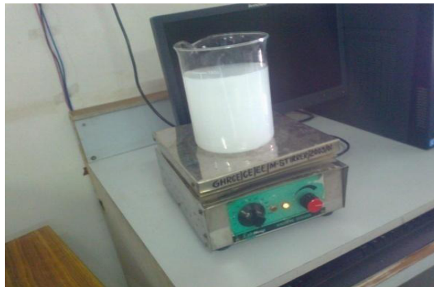
Fig 1: - Prepared nanofluid solution with magnetic stirrer
