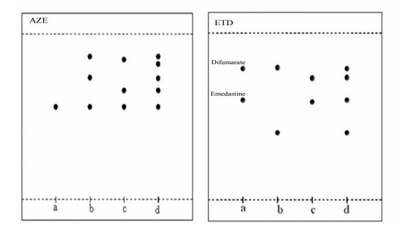
Fig. 1 Thin layer chromatogram of (a) azelastine-HCl or emedastine and their(b) oxidative degradants (c) acid degradants (d) mixture of pure and degraded drugs, developing system: methanol-10% aqueous ammonia (9.5: 0.5 v/v).
