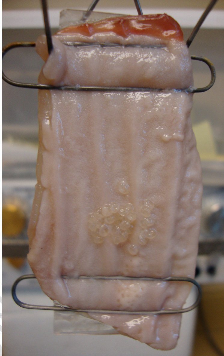
Fig. 1. Mucoadhesion testing showing pig's intestine fixed to a slide and beads adhering to it.
