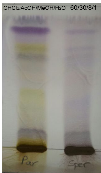
Figure 1. TLC chromatogram of crude saponins extract on silica gel sprayed with the Godin reagent. Chloroform/ Ethyl acetate/ Methanol/ Water (60: 30: 8: 1) used as solvent. Par: crude saponin extract of P. argentea ; Sper: saponin extract of S. marginata .
