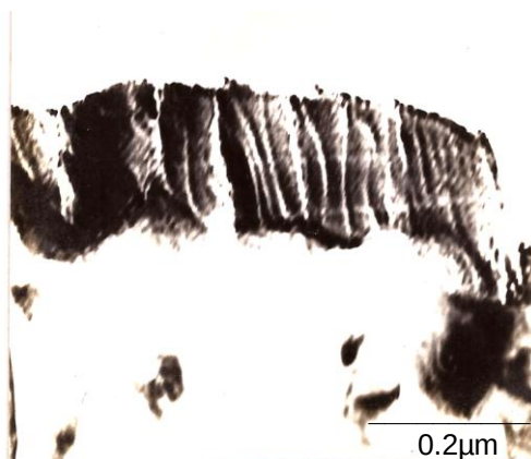
Fig.9: TEM micrograph of chromate-phosphate conversion coating without a top coating of lacquer after immersion in KCl solution for 30 days.
