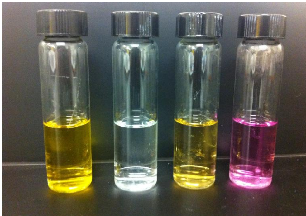
Figure 2: (Left to Right) a) Manganese Chloride b) Ferrous Sulphate c) Ferric Chloride d) Cobalt Chloride did not show any precipitation from a mixture containing both saturated and unsaturated FAs.
