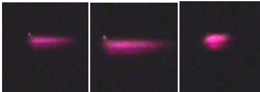
117 Fig. 3. Volt-ampere characteristics and images of the contraction of discharges at 20.9 118 Torr and 400 \mu m .
