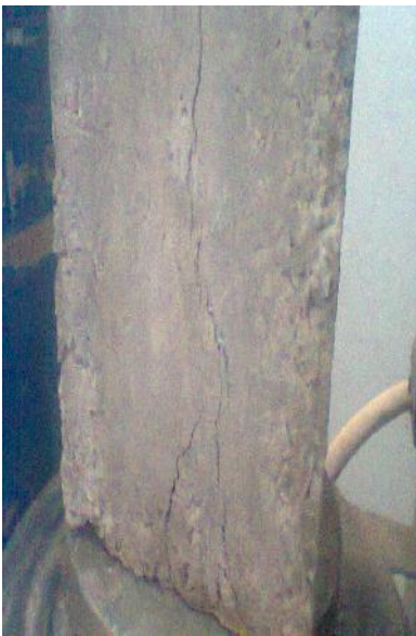
Fig.5. Failure mode in Steel Reinforced Strut
