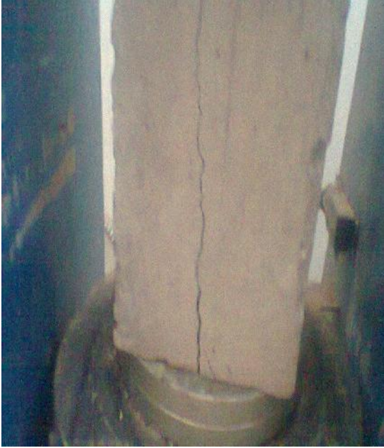
Fig.4 Failure mode in Bamboo Reinforced Strut
