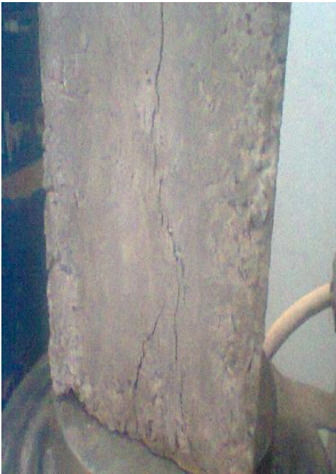
Fig.5. Failure mode in Steel Reinforced Strut
