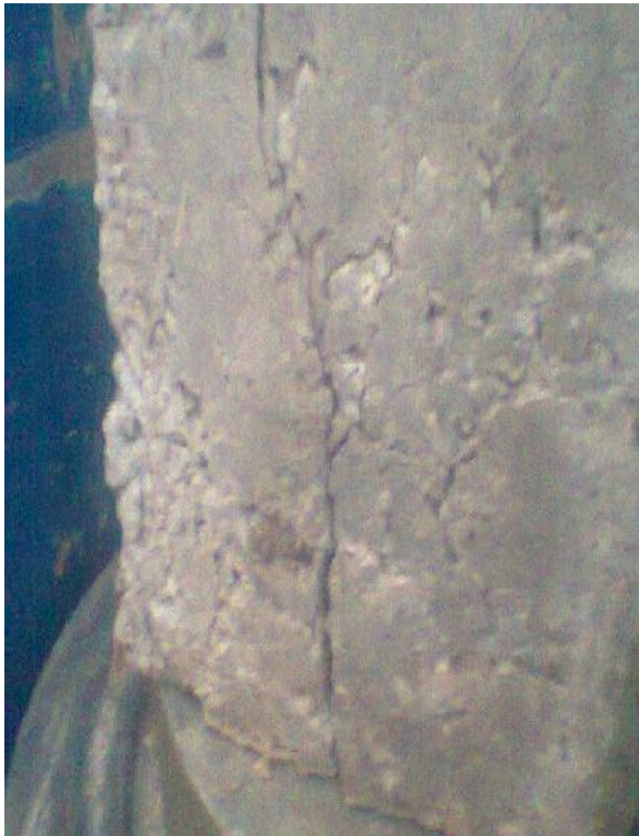
Figure 3. Failure mode in Rattan cane reinforced Strut
