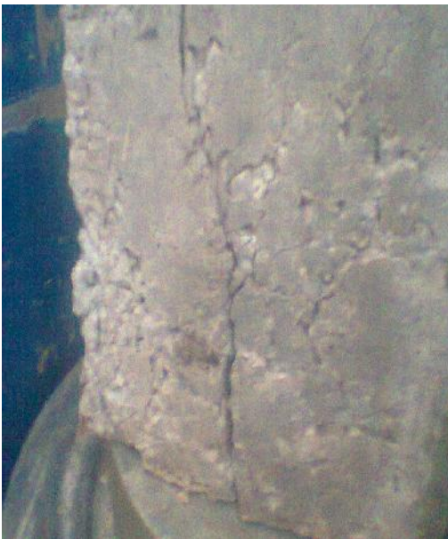
Figure 3. Failure mode in Rattan cane reinforced Strut
