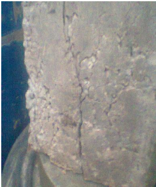
Figure 3. Failure mode in Rattan cane reinforced Strut
