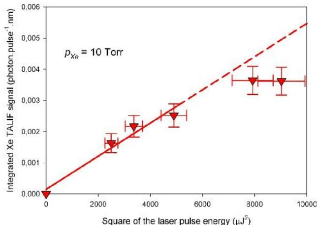
277 **Fig. 9. Integrated Xe TALIF signal versus the square of the laser pulse energy.**
