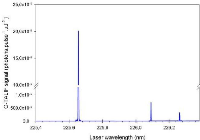
**Fig. 5. Two-photon excitation spectrum of atomic oxygen (emission wavelength: 845 nm) recorded in the plasma column in the center of the cell at 600 mbar, Air flow= 11.64 L/min, H<sub>2</sub> flow= 0.36 L/min, P<sub>MW</sub> = 1 kW .**
