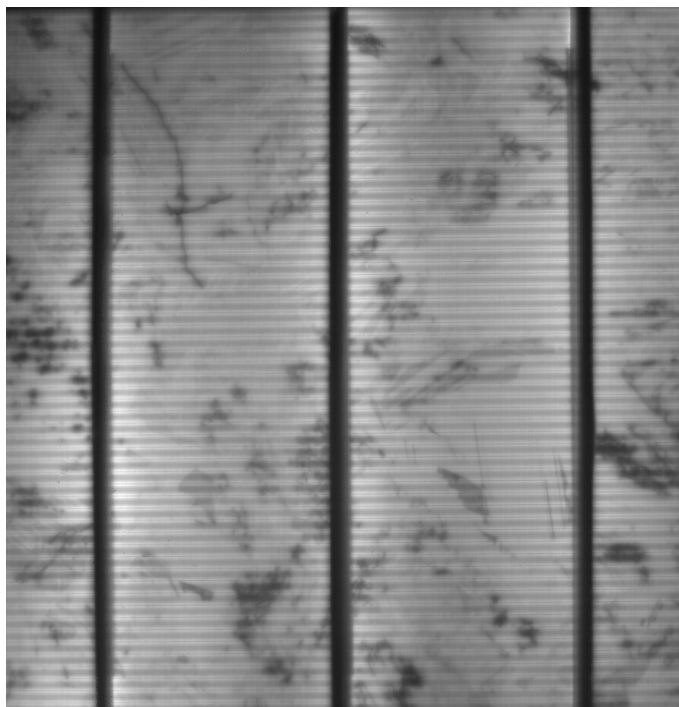
Fig. 2. Example of polycrystalline solar wafer with micro-crack
