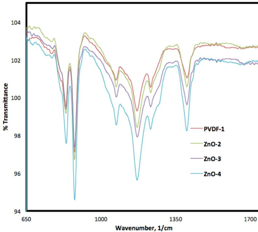
Fig 4. FTIR spectra of PVDF and PVDF/ZnO nanocomposites
