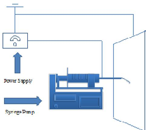
Figure 1: Experimental setup diagram. The syringe tip was connected to the power supply which delivered 10 kV DC voltage. Due to electrostatic attraction, a PbTe/silicone composite rod was extruded.
