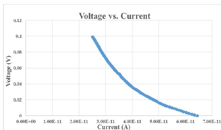
Figure 3: CHI 600E Electrochemical Analyzer supplied a decrement voltage of 0.001 V from 0.1 to 0 V.
