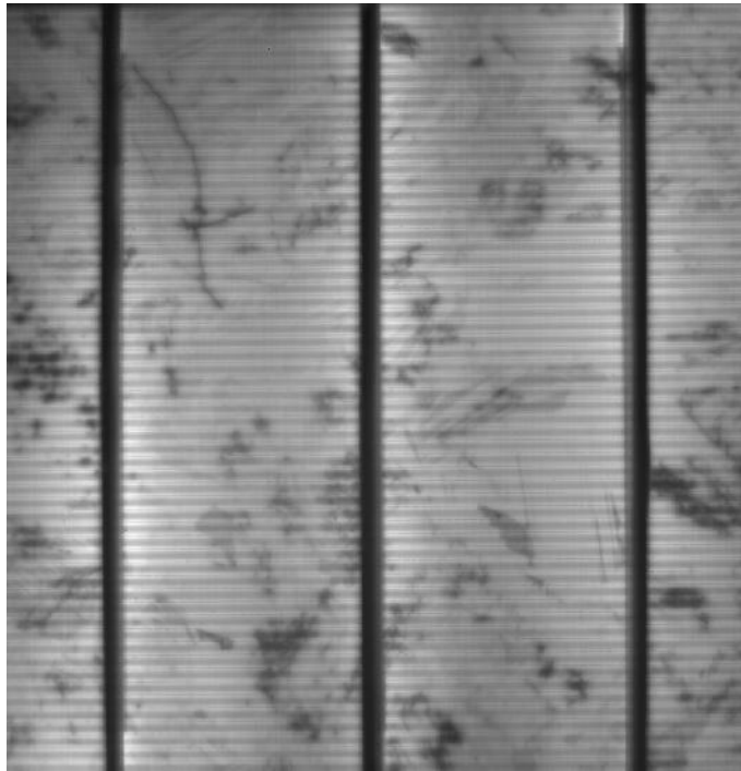
67 68 69 Fig. 2. Example of polycrystalline solar wafer with micro-crack 70
